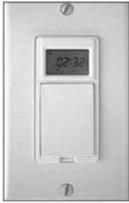
Replaces standard wall switch (toggle) to provide automatic control of outdoor or indoor lighting, fans, pumps, office machines, and other types of circuits. The unit can be programmed for 7-ON and 7-OFF events daily or weekly. SPECIFICATIONS: Input; 120VAC, 60 Hz. Switch Rating; 15A Ballast @ 120VAC, 15A Tungsten @ 120VAC, 1800W resistive.
