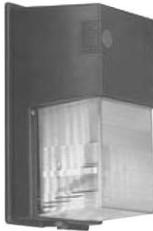
Full polycarbonate front provides vandal resistance and efficient spread. Lateral coverage is 5 times the typical mounting height of 6-10 feet. Molded-in bronze finish. UL Listed for use in wet locations. Lamp included.
