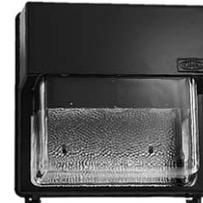
Clear borosilicate glass lens allows shielded lamp to direct main beam downwards. Shielded lamp above a specular hammertone reflector provides beam control, socket is adjustable for deeper shielding. Dark bronze power paint finish. CSA certified for use in wet locations.
