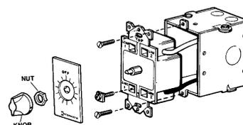
Designed to be used with standard or decora style switch plates. This spring wound, manually set, time switch automatically turns "Off" ventilating fans, heaters, heat lamps, lights, and can operate as a thermostat bypass. Rating: 20 amps, 125VAC, 1 HP; 10 amps, 250VAC, 1 HP; 10 amps, 277VAC; 7 amps, 125VAC tungsten rating S.P.S.T. Mounts in standard 2-1/2" deep switch box.
