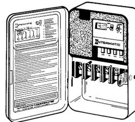
Easy to operate solid-state digital electronic timer. All programming and clock setting is accomplished with the use of two slide switches and four/five pushbuttons. Comes with factory installed industrial grade standard "AA" alkaline battery to provide timekeeping and automatic carry-over for a minimum of 3 years. 120V clock supply. 30A per pole. Indoor rated enclosure.
