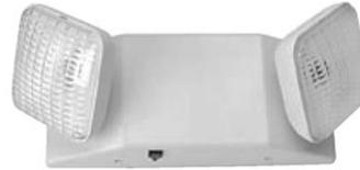
Universal J-box mounting with quick-connect adapter for fast, simple installation. Compact, low profile design. Fully automatic operation. 6-volt premium grade, lead-acid, maintenance-free battery with 10 year expected life. 120/277 VAC operation. Thermoplastic white housing.
