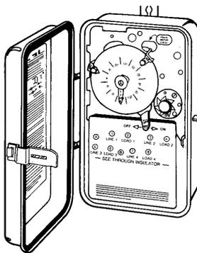
Standard "On-Off" time switches. Has the same applications and performs functions similar to the T100 time switch, plus it allows you to omit operation on Saturday, Sunday or any other selected day(s) of the week. All models equipped with one Cutout Tripper (which also serves as "On" tripper), one "Off" tripper and three skipping screws. 40 amp resistive or inductive each pole, 120-480 volts AC.
