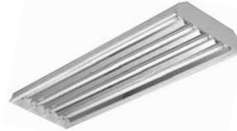
High efficiency T5 & T8 lamps for significant energy savings over HID high bays. Unit may be pendant, chain or surface mounted. Shallow fixture dept 3-7/32". Minimum fixture weight - less load on building structure. Less lamps.
