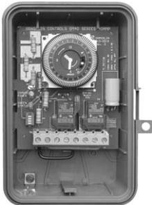
The GM40 Multi-Volt Series Time Controls are universal, electromechanical time switches which can be field configured for various power supply voltages. The voltage options include 120VAC, 208/240VAC, and 277VAC. Compact NEMA 3R outdoor enclosure features a DPDT switching configuration.
