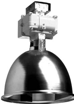
Field adjustable lighting distribution patterns and rugged construction make this fixture ideal for new construction or quick and easy retro-lighting of existing systems. Will accommodate mounting heights as low as 12' to as high as 30'. 3/4" pendant mount. New quick-on mounting permits one man installation. Furnished with quad tap HPF ballast; 120, 208, 240, 277V. Less lamp.
