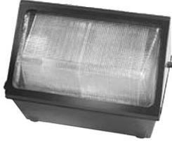
Borosilicate glass refractor. 4 times spacing to mounting height. All units have dark bronze powder paint finish, Quad-Tap® ballasts and lamps included. UL Listed for use in wet locations.
