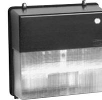
One piece polycarbonate lens, internally painted for lasting appearance. 6 to 1 spacing to mounting height ratio. Housing is die cast aluminum. Specular reflector, vertical lamp and refractor combine for efficient and uniform perimeter lighting. CSA certified for use in wet locations. Lamp included.
