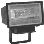
A compact H.I.D. floodlight for energy efficient outdoor light. Utilizes all of the efficient H.I.D. sources, including High Pressure Sodium and Metal Halide. Includes 2 bolt steel trunion with center hole for nipple mount. Bronze powder coat protective finish. Wide, uniform beam for illumination of signs, facades and larger areas. Coverage is four times set back distance. Lamp included. CSA certified to UL 1598. Yoke mount.
