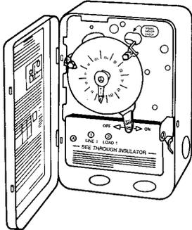
Standard "On-Off" time switches. Provides 1 to 12 "On-Off" operations every day, depending on number of trippers used. Allows timing of 1 to 23 hours. One "On" and one "Off" tripper furnished with each switch. 40 amp. Resistive or inductive each pole, 120-480 volts AC.
