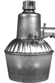
Luminaire package consists of a universal die cast head and ballast, acrylic open bottom refractor, photoelectric control for 120V circuit, 1-1/4" x 24" pipe bracket, and either a 100W HPS or 175W mercury lamp.
