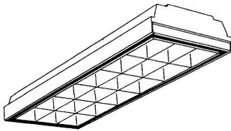
High efficiency, T8, parabolic. 120/277V. Energy efficient ballast. 3" deep louver - spring loaded latches and T-hinges.
